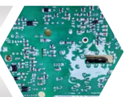
三防&保护 Coating & protecting
